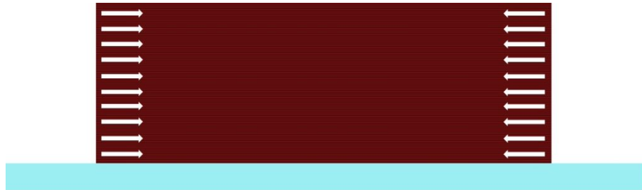
Figure 21: Printed part which has just finished printing, the part and the build-plate are roughly at the same temperature. The part is already exerting some force as a result of shrinkage during the solidification of the deposited FDM thermoplastic
