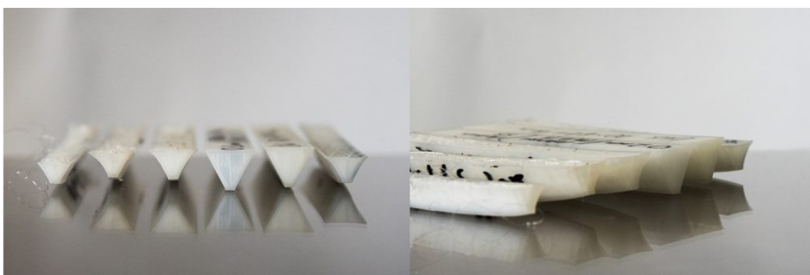
Figure 29: Prints using the same material warping to different extents when being printed at different bed temperatures.
