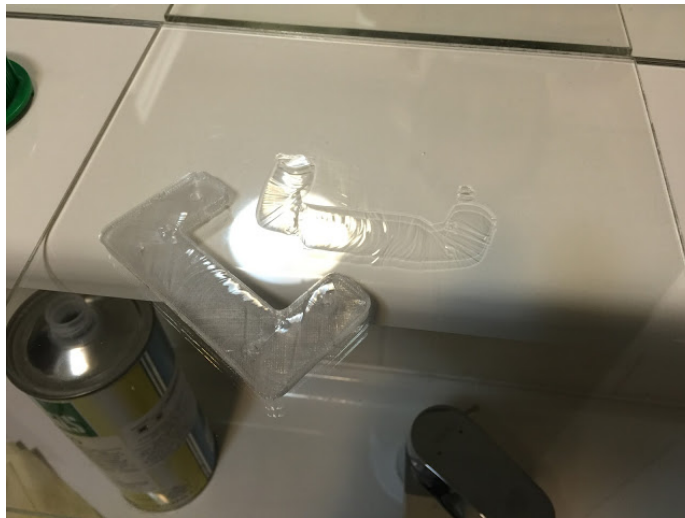
Figure 24: A PET-G print causing a catastrophic failure on a glass build-plate, image via richrap.blogspot.com
