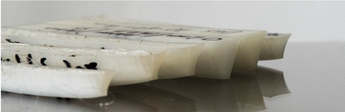
Figure 14: Wedge prints at different temperatures showing different amounts of warp and/or rates of completion
